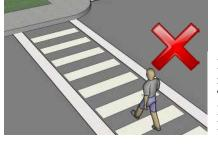
If existing pavement markings such as linear stripes are present, it is mostlikely that the pavement will have to be removed and replaced. These heavy markings cannot be removed from the surface without leaving unsightly marks (ghost lines). One may consider applying DuraTherm over very faint markings.
