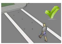
Minor amounts of oil droplets (up to 10 small spots less than 2 inches in diameter per 300 sq. ft.) are acceptable and should evaporate during the heating process. If small spots are more frequent, power washing should be done prior to application.
