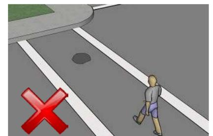
If larger areas are contaminated by oil, then they must be removed by power washing. If the oil is soaked in and cannot be washed away, then the pavement must be removed and replaced.
